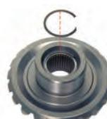
Forward gear has retaining
